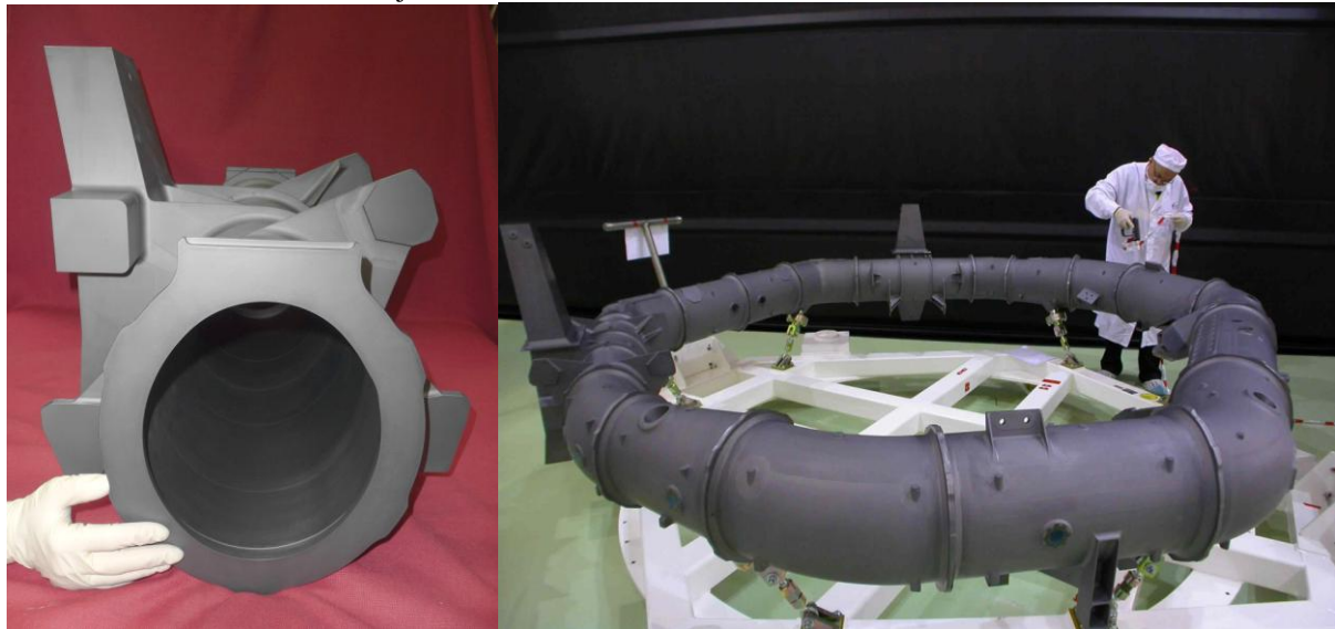
Fig. 4. Torus Left ) Torus segment before brazing Right ) Reception of the torus assembly in Astrium (< 200 kg)
