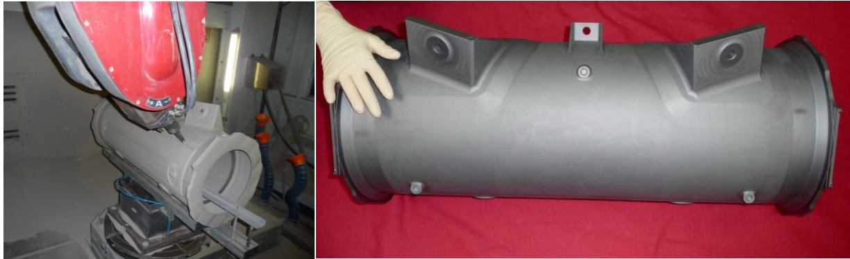
Fig. 2. One of the 19 GAIA torus segments ( left ) during green machining, ( right ) ready for brazing assembly
